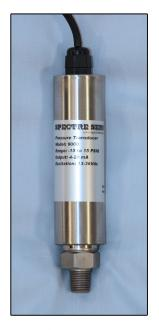
Spectre's Series 9000 is the first available pressure transducer that is designed, manufactured and calibrated to each application's specific operating conditions. *Each transducer's output is digitally mapped to correct for any non-linearity or inaccuracies in the sensing element.* This digital correction provides the most accurate and flexible pressure transducer in the industry.
